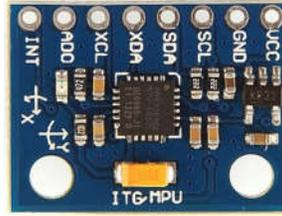
Fig.7 MPU 6050 Accelerometer and Gyroscope (source [19] [www.arduino.cc](http://www.arduino.cc))
