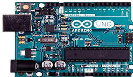
Fig.6 Arduino UNO (source [19] [www.arduino.cc](http://www.arduino.cc))
