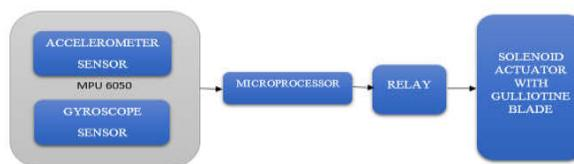
Fig.2 Block diagram of Proposed system
