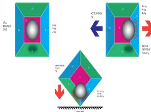
Fig.9 Accelerometer Working ( source [17] [www.classes.engineering.wustl.edu](http://www.classes.engineering.wustl.edu))
