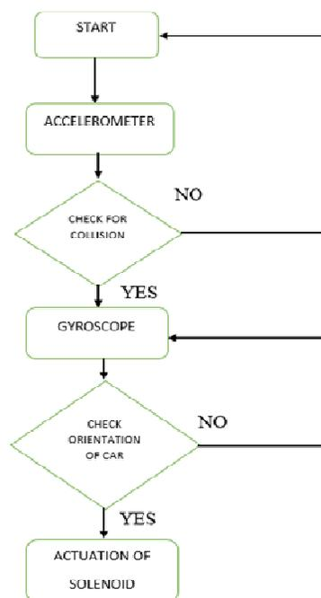
Fig.4 Algorithm used in Proposed system
