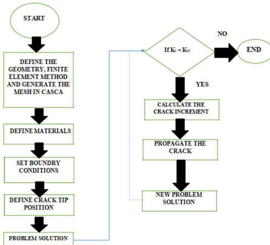
Figure 1 Flow chart of crack propagation approach in FRANC-2D
