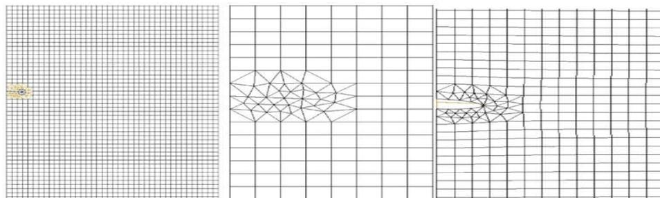
**Figure 4** Crack initiation at crack flaw and deformation crack area meshing
