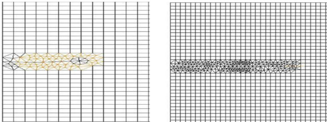
Figure 7 Meshing of the crack propagation region
