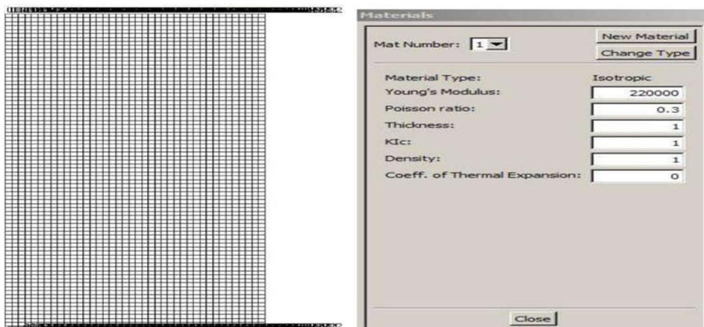
Figure 3 Definition of load distribution and material properties in FRANC-2D
