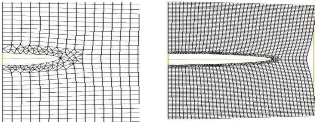
Figure 9 Deformed Mesh with crack Propagation region
