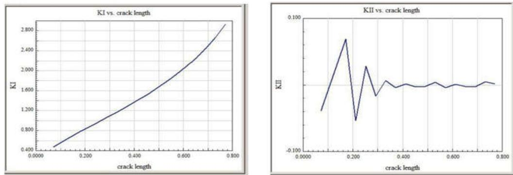
Figure 11 FRANC – 2D crack length versus stress intensity factor plots
