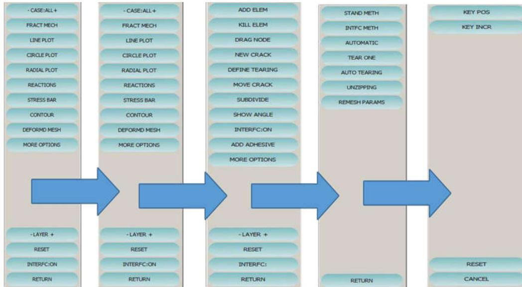
Figure 6 FRANC-2D simulation steps involved for crack propagation
