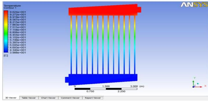
Fig. 8 Temperature distribution
