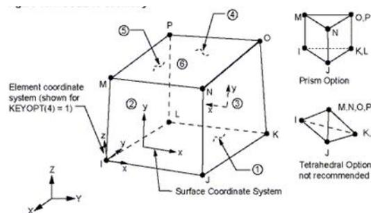
Fig. 2 SOLID45 Geometry
