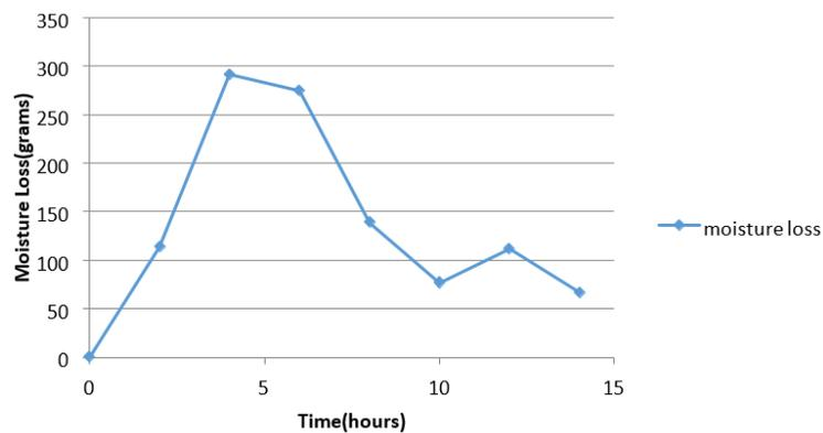
**Figure 26** Moisture loss from the product versus time
