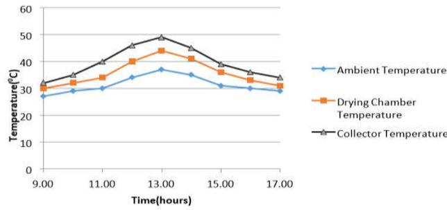
Figure 9 Variation of temperature versus time for sample 1 on day 2
