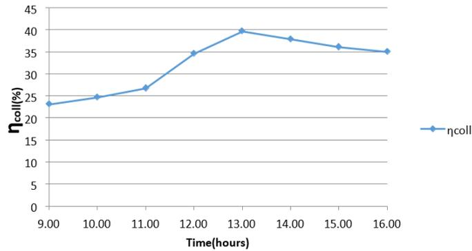
Figure 23 Collector efficiency versus time for sample 2 on day 2
