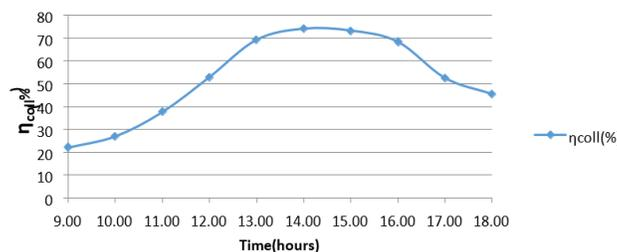
**Figure 8** Collector efficiency versus time for sample 1 on day 1
