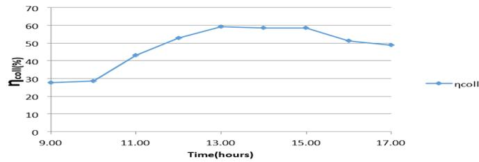
Figure 10 Collector efficiency versus time for sample 1 on day 2
