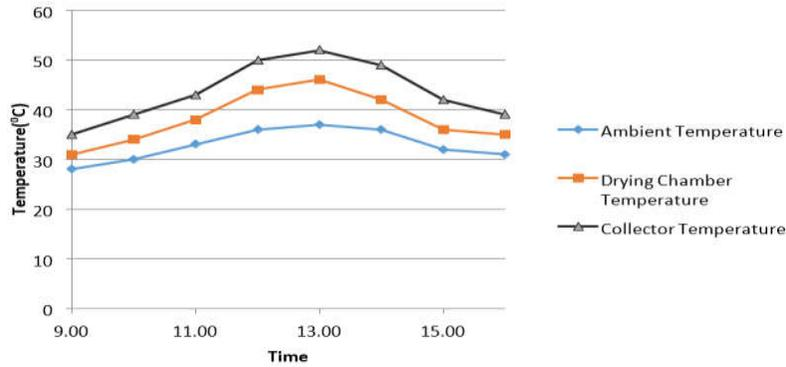
Figure 22 Variation of temperature versus time for sample 2 on day 2
