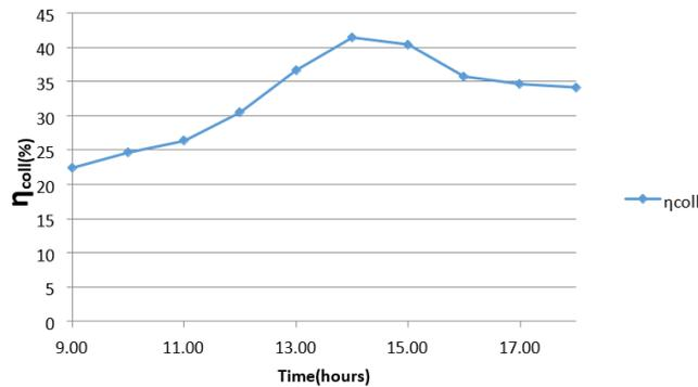
Figure 21 Collector efficiency versus time for sample 2 on day 1
