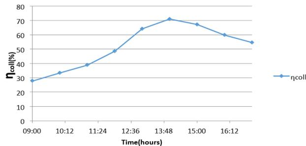
Figure 12 Collector efficiency versus time for sample 1 on day 3
