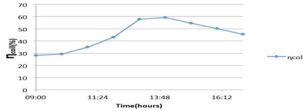
Figure 14 Collector efficiency versus time for sample 1 on day 4
