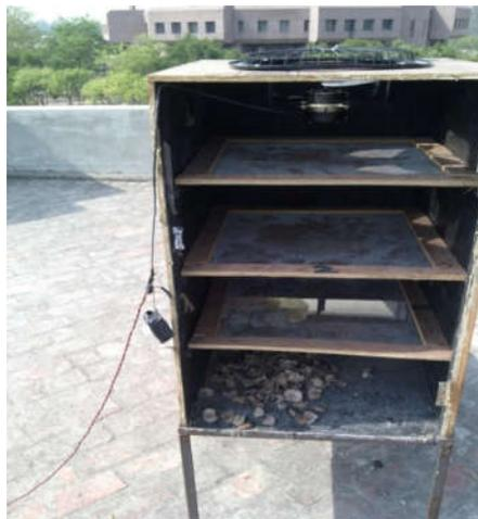
**Figure 2** Drying chamber
