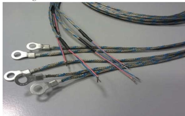
Figure 5 J-type thermocouple
