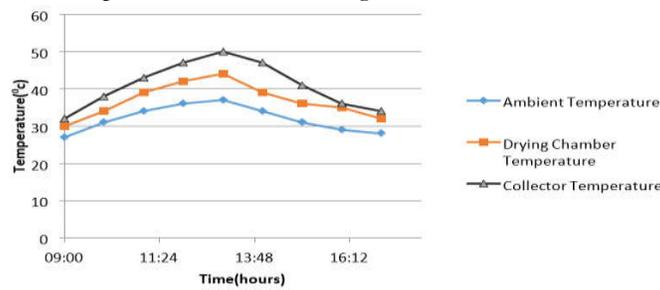
Figure 11 Variation of temperature versus time for sample 1 on day 3
