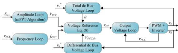
Fig 2.3 the proposed control technique with plenitfulness and repeat Frequency loops.
