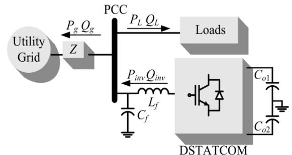
Fig. 1.1 A Low voltage distribution grid at under analysis with voltage controller.
