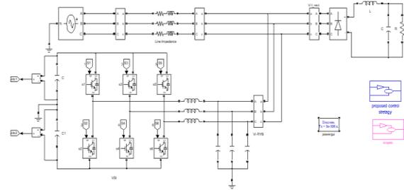
Fig 3.7: Dstatcom Compensator with Non Linear Loads
