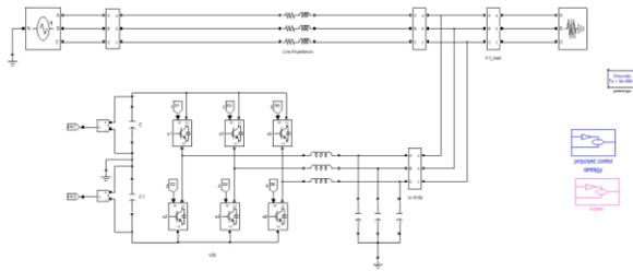
Fig 3.3: Dstatcom Compensator with Linear Loads
