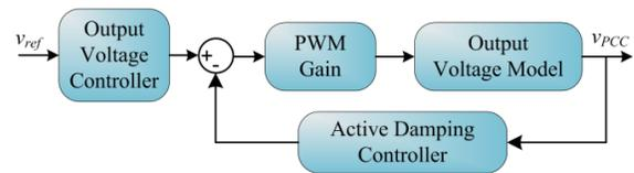
Fig. 2.4. block diagram of the output response voltage loop
