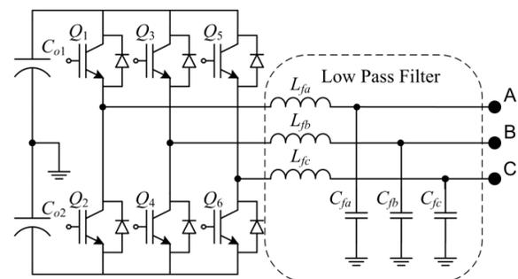
Fig 2.1. LC low-pass filter with 3- $\Phi$  4 wire VSI
