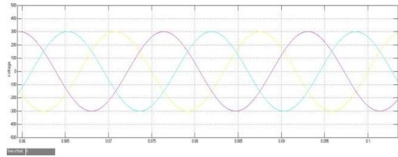
Fig 3.16 Linear Loads With Dstatcom Compensator Waveforms
