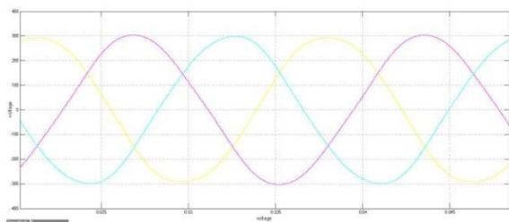
Fig 3.6 Linear Loads Without Dstatcom Compensator Waveforms
