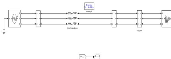
Fig 3.5 Linear Loads without Dstatcom Compensator
