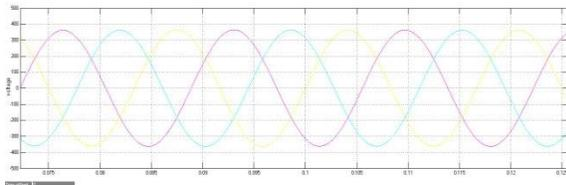
Fig 3.18 Non Linear Loads With Dstatcom Compensator Waveforms
