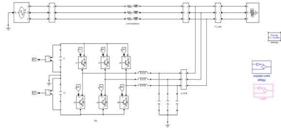
Fig 3.15 : Linear Loads With Dstatcom Compensator
