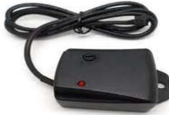
**Fig.2.1.2: Vibration Sensor**
