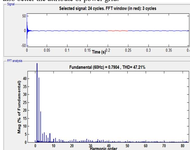
Figure 2. harmonic analysis with 48 pulse statcom
