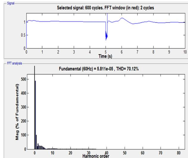
Figure 1. harmoni analysi with 12 pulse statcom
