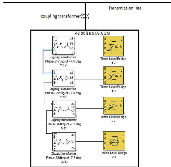
Figure1. 48 Pulse Static Synchronous Compensator (STATCOM)
