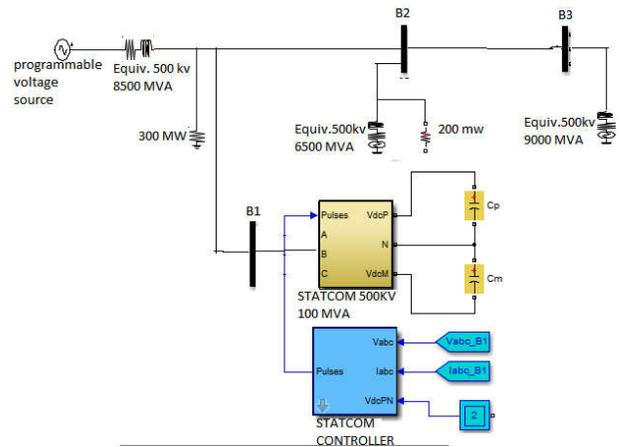
Figure 2. System with 48 pulse STATCOM
